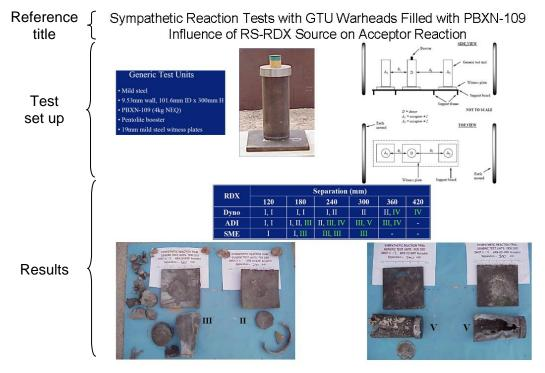
Figure 7: Example of Pictures Describing Test Set-Up and Results (SYR v1.2)
