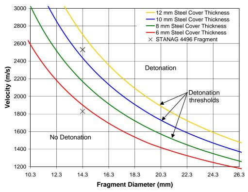
Figure 14: TEMPER Simulation of STANAG 4496 Fragment Impact on PBXN-110 Blocks Covered with Steel
