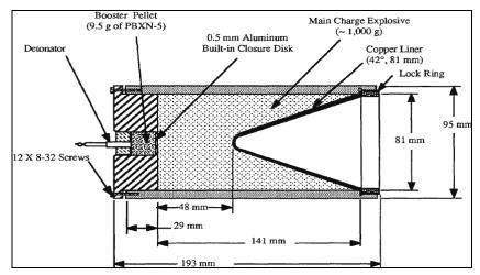
Figure 4: Example of GTU Drawing - 3.2" Generic Shaped Charge Testing Unit (BIRD v1.2)
